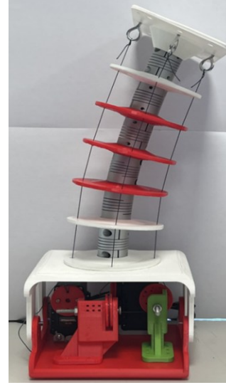
Fig.6. LARMbot humanoid design, [16-18]: a) inspiration from the human musculoskeletal anatomy; b) tripod architecture for limbs; c) serial-parallel mechanism for the torso; d) a CAD design of the full assembly
