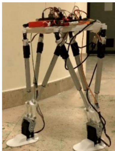
Figura 5: LARMbot humanoid robot: substructures under development for dual arm unit, torso unit, and leg unit
