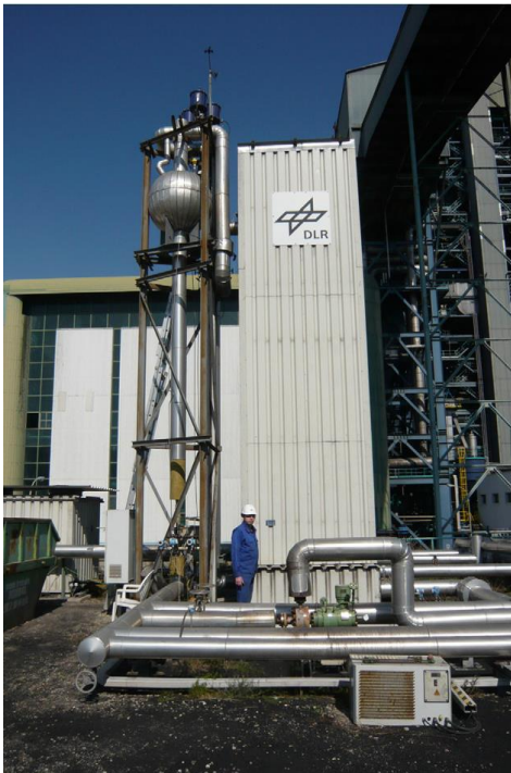
Experimental demonstrator of latent heat storage (sodium nitrate) with a capacity of 700 kWh
