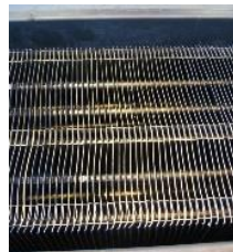
Finned Tube Design effective thermal conductivity >10 \text{ W/(mK)}
