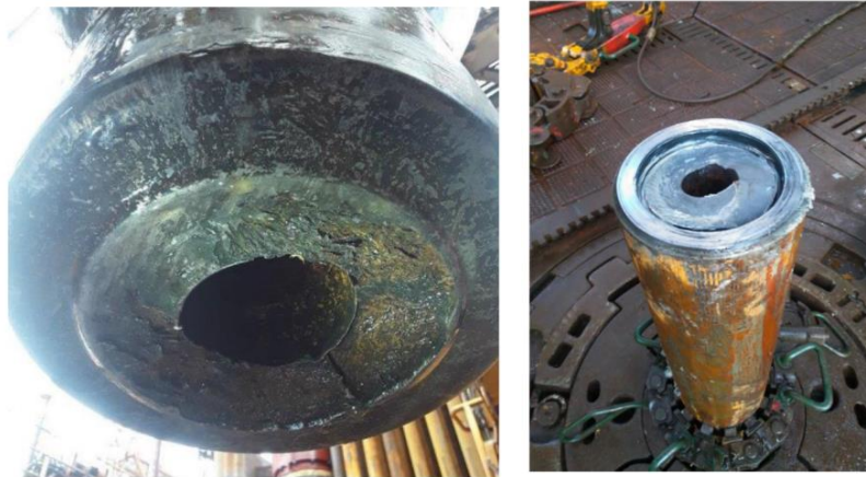
Figure 12 - On the right, the broken pin between the sub and stabilizer. In the left, the broken pin in the connection of the Drilling Jar.
