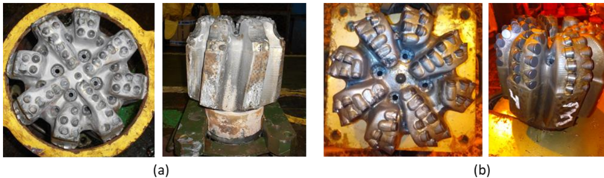
Fig. 2—Comparison of (a) typical dull bit used in the reservoir section, and (b) dull bit used to drill the last well in Lapa Phase 2.
