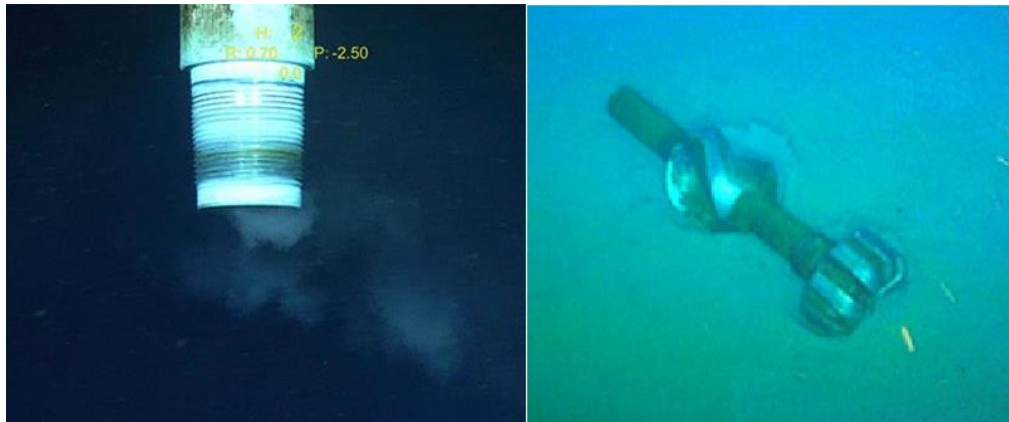
Figure 10 - The pin from the second disconnection point and the Near Bit with the drill bit on the seafloor
