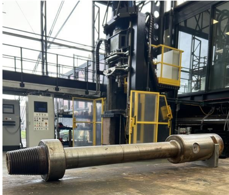
Fig. 3—LAM with the compliant HFTO-enabling shaft.
