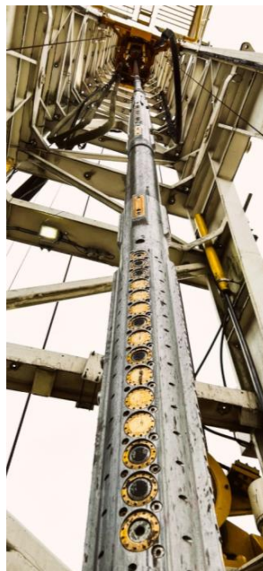
Figure 7 – CP suspended in derrick during drilling tests at drilling contractor facility, Houston, TX
