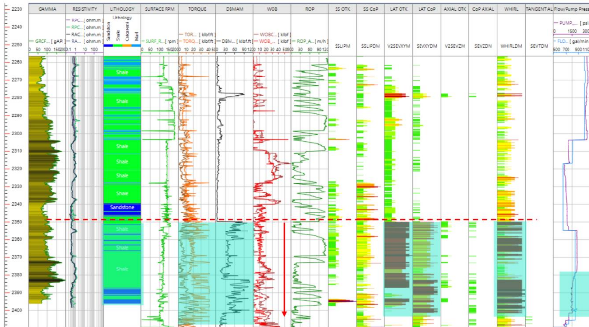
Figure 13 – Drilling and Vibration parameters during Well A section
