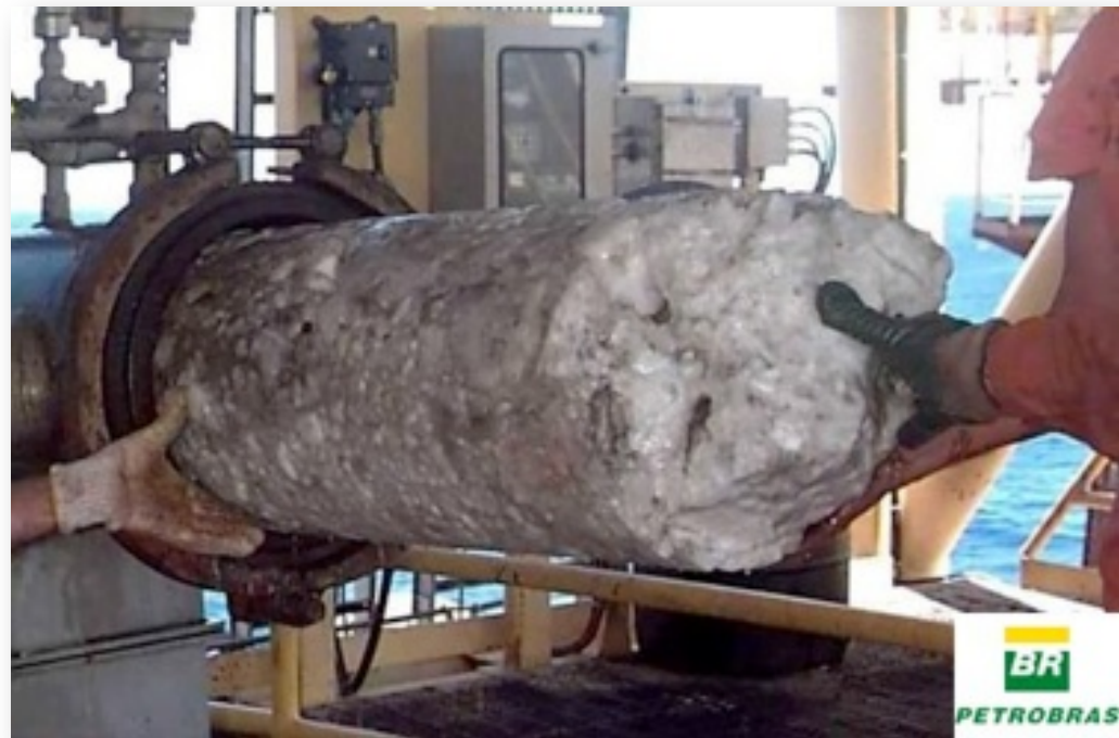
Hydrate plug removed from oil pipeline
