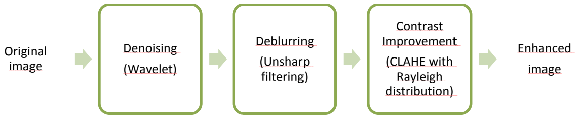
Figure 13. Flowchart of the proposed enhancement algorithm
